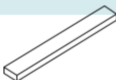
Flexural testing specimen GB/T 9341
