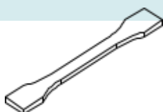
Tensile testing specimen GB/T 1040
