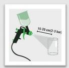
Apply AESUB green from a distance of 15-20 cm with a spray gun. We recommend either the battery-operated AESUB spray gun (AESSG001) or spray guns with a nozzle diameter of 1 mm or more. Spray the complete surface to be scanned.
