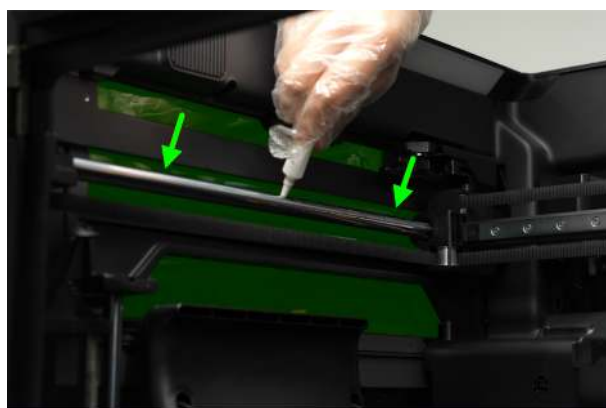
Lubricate the left Y-axis rod
