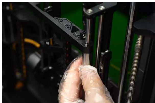
Lubricate the linear rods
