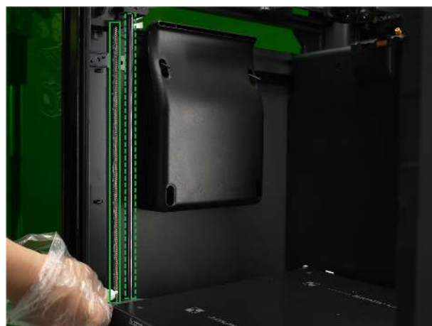
Lubricate the Z-axis lead screws and linear rods
