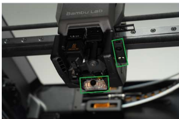
Clean the toolhead camera and nozzle camera
