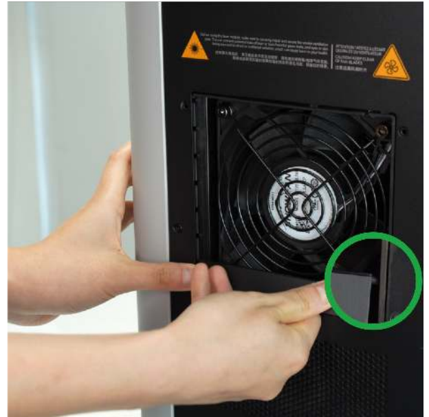
Snap the right positioning block into the slot
