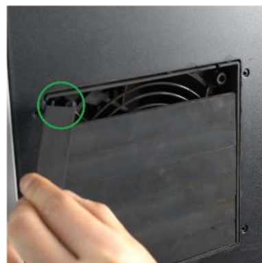
Lift the latch upward to remove it
