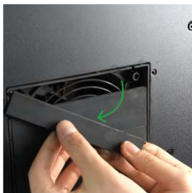
Rotate 90° clockwise to remove
