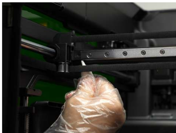
Lubricate the lower side of the X-axis linear rail
